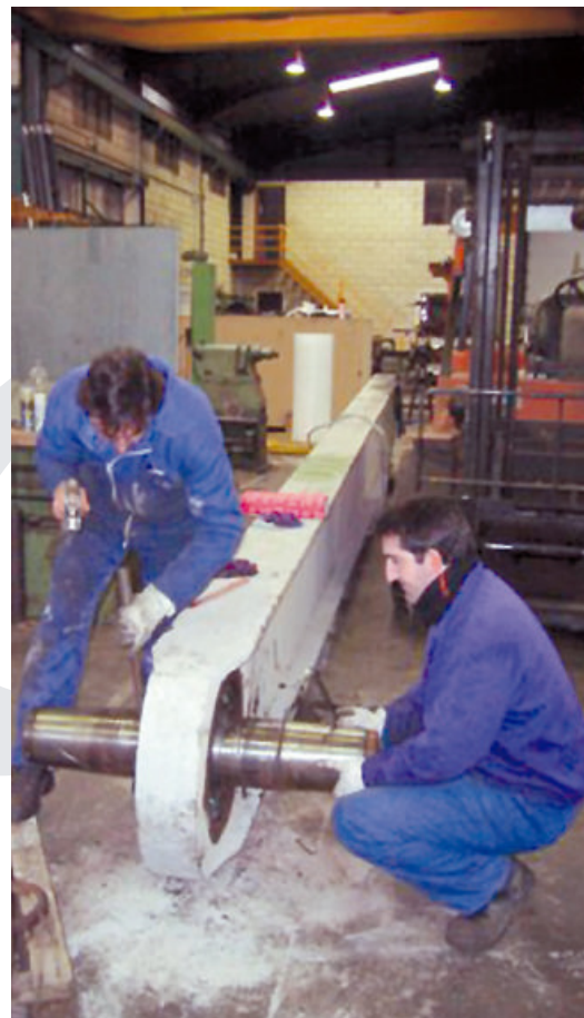
REPARANDO BIELA / REPAIRING CONNECTING ROD
