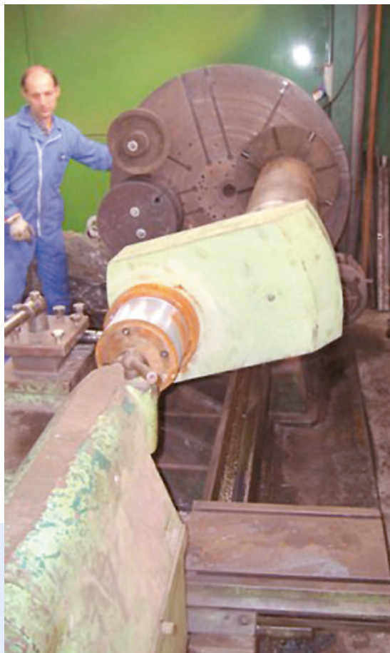
REPARANDO BIELA / REPAIRING CONNECTING ROD
