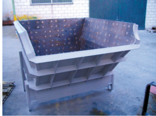
TOLVA ANTIDESGASTE ANTI-WEAR HOPPER
