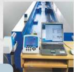
Straightness inspection with collimator
