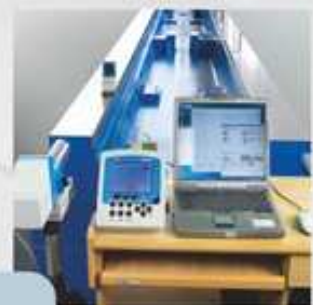
Straightness inspection with collimator
