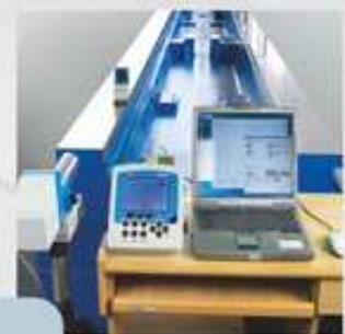
Straightness inspection with collimator
