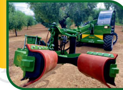
Rulli in gomma con mescola esclusiva Sicma Rubber pillows with Sicma exclusive mixture
