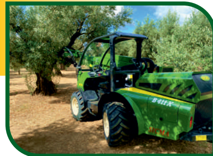
Trazione idrostatica indipendente sulle 4 ruote e assale sterzante posteriore Independent and hydrostatic 4-wheel drive with rear steering axle
