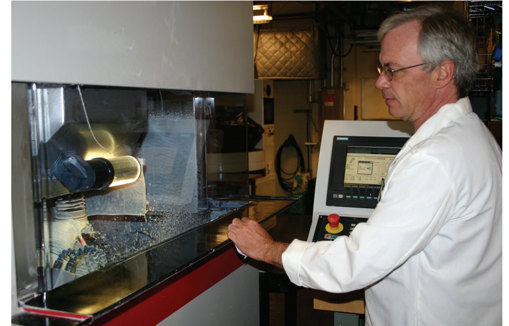
A II-VI Infrared optician operating a CNC polishing machine.
