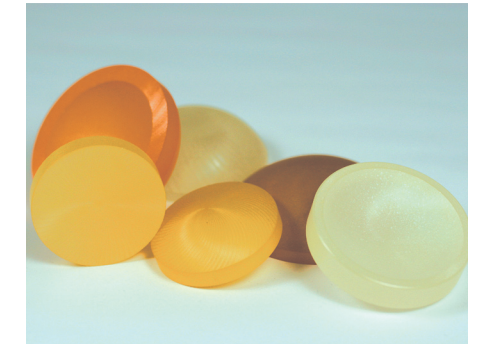
Figure 5 Generated curved lens blanks
